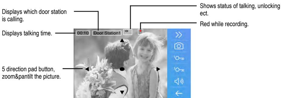
**Note:** The 5 direction pad operation should make effective with **fish-eye** door station.
